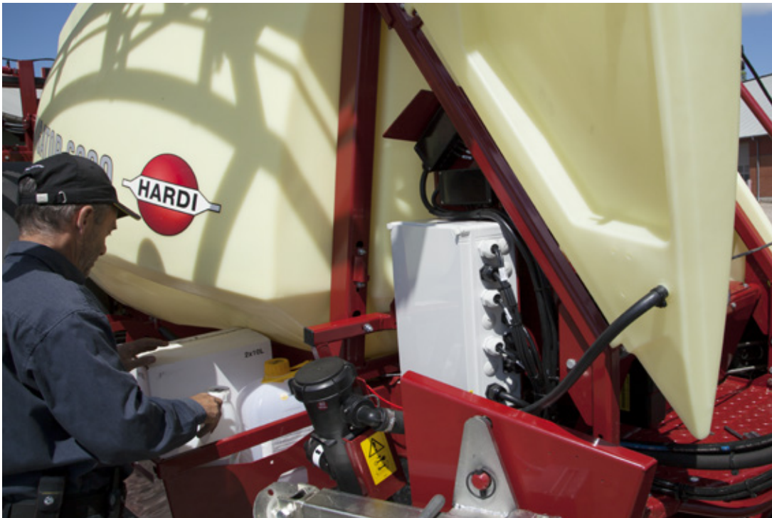
HARDI ECU containing ISOBUS Bridge and JobCom.
