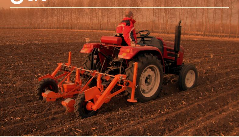
Used all over the world the 870 is the market leading belt planter. With a 7 speed pulley drive courtesy of adjustable height landwheels, the 870 can work on the flat or bed setups. Available from 2 rows up to 18 rows and capable of multiline planting, the 870 is robust, scalable and adaptable for every seed type.
